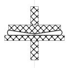
We have to measure viscosity of material. Easiest this is done by a dynamic cone-plate rheometer to get a complex viscosity flow curve as a function of frequency. In principle there is also possible to use other devices and methods.
